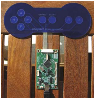
Capacitive touch USB joystick. Engineers using the Rapid Keypads configuration utility can map custom capacitive touch buttons to any key on their computer keyboard, numeric keypad, or computer joystick. Image courtesy of RapidKeypads.com.
